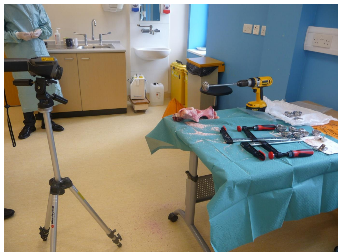
Figure 2 - Hemi-pelvis and FLIR E45 camera position during testing. Note reamer on the end of the drill and some debris from reaming process
